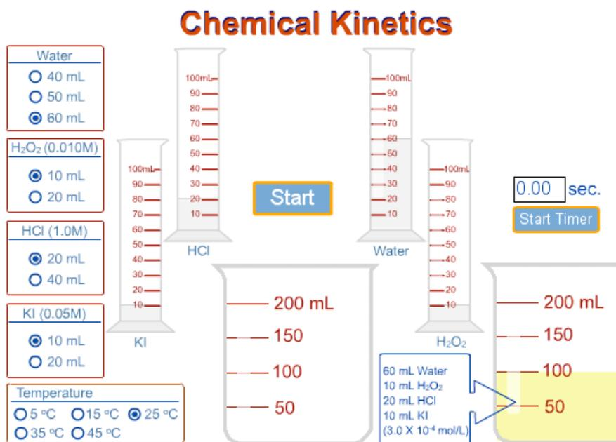
The reaction to be investigated occurs in the beaker when four colorless solutions from four graduated cylinders are mixed. Different amounts of the solutions can be added together at different specified temperatures. Radio buttons control these amounts and the temperature. A timer can be used to monitor how long it takes for the chemical reaction to proceed to the same level of completeness as the standard solution contained in a second beaker.
